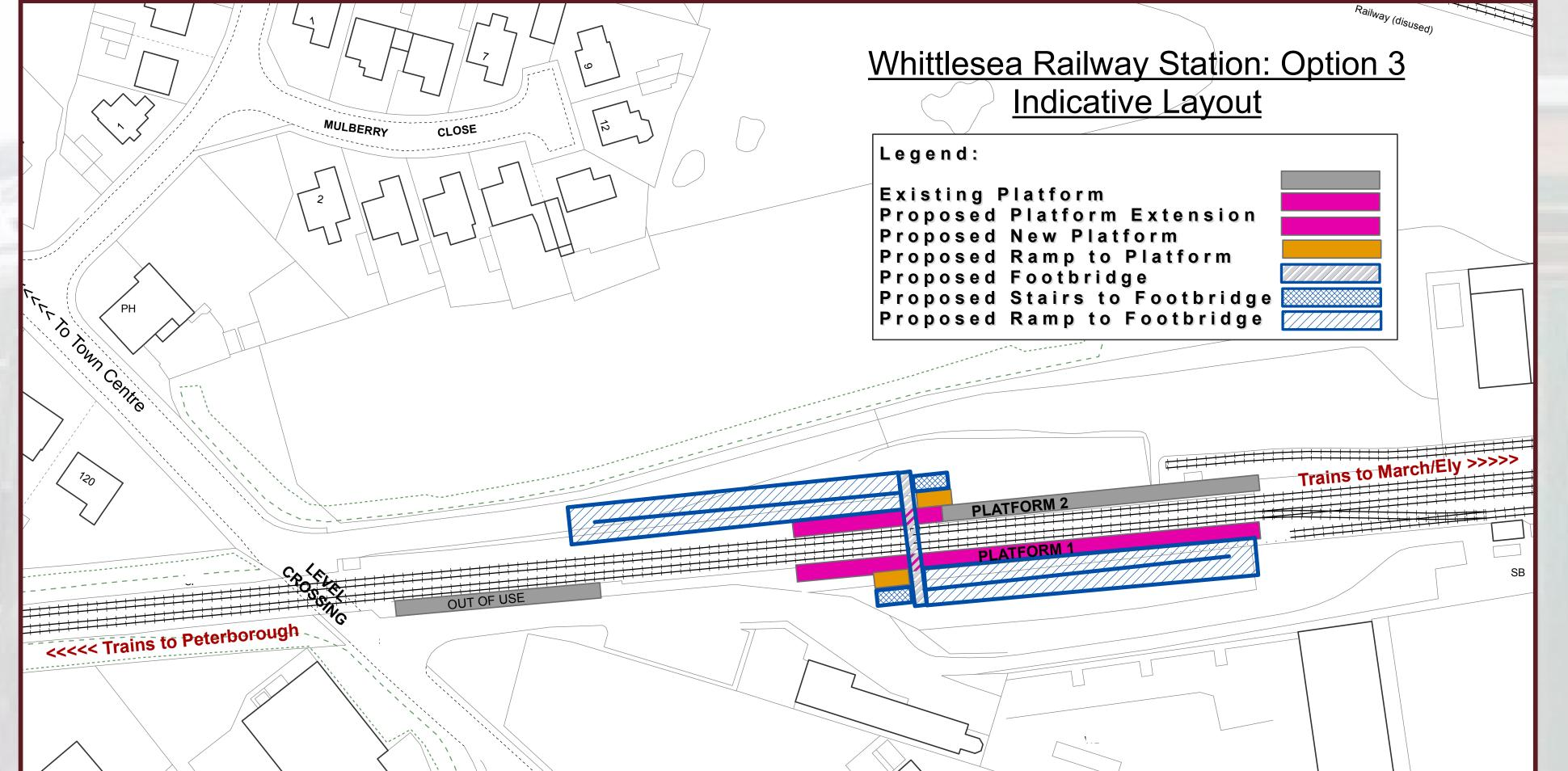
This option does change the existing station layout by creating a new Platform 1 opposite Platform 2. However, this does reduce the overall footprint of the station. The siting of Platform 1 is further away from Station Road than the other options. This could cause a slight increase in the time the level crossing is closed.
